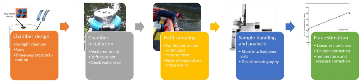
Figure 1. Measurement procedure of greenhouse gas fluxes from shrimp farms using floating chambers
